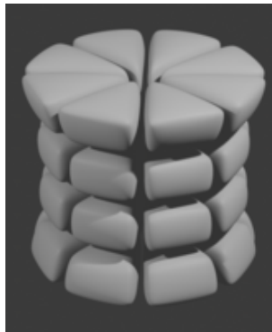
Figure 1.11: Schematic of a fuel pellet with a “hourglassing” shape due to the effect of thermal stresses
